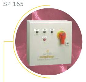
Citel's SurgePurge 165 model provides highrisk surge suppression capability at your facility's *service entrance for both conducted (10/350µs)* and induced (8/20µs) transient overvoltages originating from such sources as lightning strikes and utility switching. These protectors incorporate Citel's reliable ihigh intensity modules with individually monitored and fused MOVs. Designed to various national and international standards the SurgeGuard is ideal as a global protection solution.
