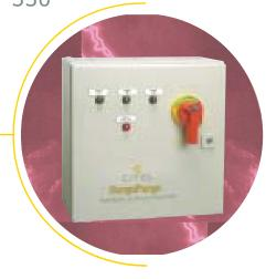
Citel's SurgePurge 330 model pr margine surge suppression capability for your facility's service entrance for both conducted  $(10/350\mu s)$  and induced  $(8/20\mu s)$  transient overvoltages originating from severe lightning and utility switching events. These protectors incorporate Citel's reliable ihigh intensity modules with individually monitored and fused MOVs. Designed to provide rugged, high quality surge protection at the most critical points within a facility's distribution system.
