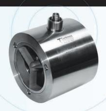
face flanges and is robust enough to handle up to 3,700 PSI, depending on the chosen flange size. The WM Series meter is unique in that rather than snap rings holding the internals, three (3) machine screws hold each rotor support in place, making this a heavy duty meter for most any liquid application.
