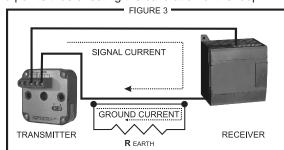
It is apparent that we are "fighting a losing battle" thinking we can anticipate the interactive affect of ground loop currents on our measurement loop. What can we do to get around this problem? The answer is to provide DC isolation between each component in our loop. (Figure 4)
