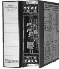
The DM4051 provides an isolated output voltage or current proportional to a differential input signal from a strain gauge(bridge) input. It is useful for measuring outputs of load cells, pressure transducers, and strain gauge sensors.
