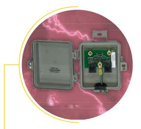
Designed to protect Power-Over-Ethernet (POE) (Mode B) network devices installed outdoor. The C2MJ8-505-RJ is designed to handle transmission speeds up to 100 BaseT. All eight pins are protected by a carefully designed circuit that isolates data from ethernet power lines. The ultra-sharp clamping response permanently eliminates transients from your outdoor POE applications.
