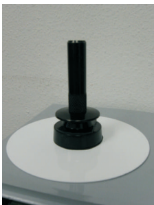
1/4 wave antenna with ground plane
