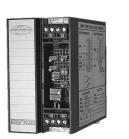
The DM4051 provides an isolated output voltage or current proportional to a differential input signal from a strain gauge(bridge) input. It is useful for measuring outputs of load cells, pressure transducers, and strain gauge sensors.
