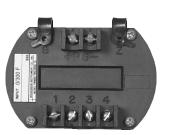
The SR8401 regulates the current in a twowire current loop to be proportional to input from a thermocouple temperature sensor. The transmitter's output is linear with the thermocouple's voltage and is compensated automatically for "cold junction" temperature changes at its input. The transmitter input and output are transformer isolated.
