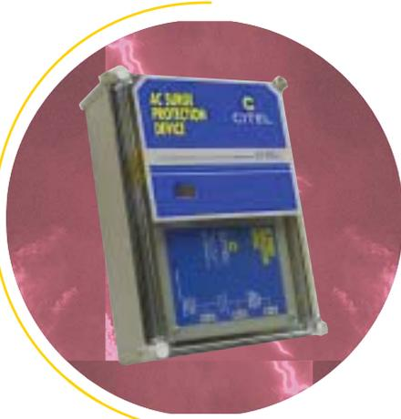
The CM80 Series is a high performance surge protector designed for critical panel locations. The SPD incorporates high-energy MOVs with EMI/RFI noise filtering to provide protection against transients originating from induced lightning strikes and utility switching.
