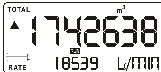
Fig. 3: Example of low-battery alarm.
