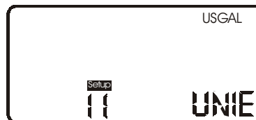
Fig. 5: Example of sub-function 11: unit for Total.
