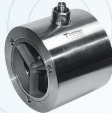
face flanges and is robust enough to handle up to 3,700 PSI, depending on the chosen flange size. The WM Series meter is unique in that rather than snap rings holding the internals, three (3) machine screws hold each rotor support in place, making this a heavy duty meter for most any liquid application.
